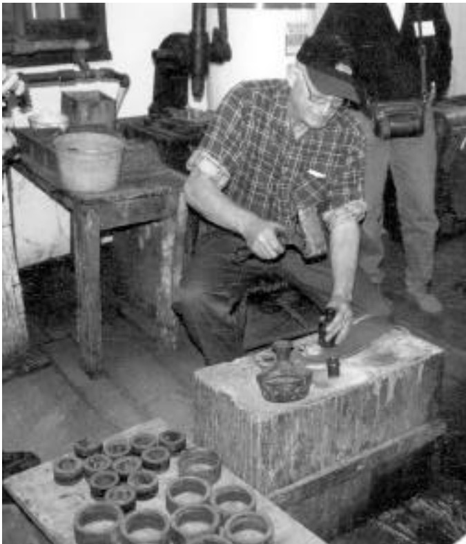
Albert Baines punches out a pump-valve cup at the Baines Machine & Repair Works. The Baines shop has been manufacturing and repairing pumps used in Petrolia's oil wells since 1914. Most of the shop's belt-driven equipment dates to its founding.
