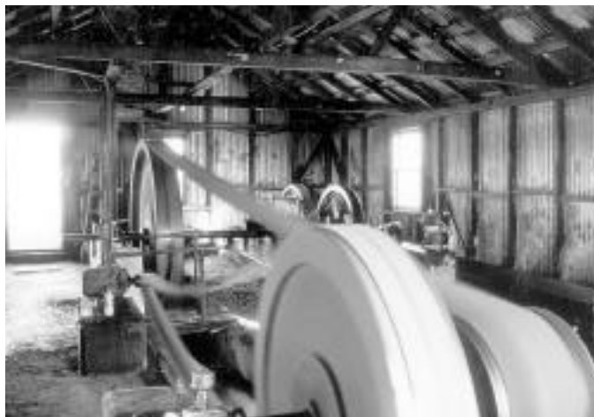
Interior of a pump house at the Fairbank Oil Properties. Thirty-odd pumps are driven by a 3-hp electric motor via belting and reduction gears.
