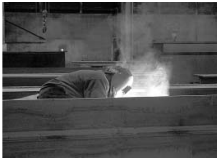
Au Dragon Forgé offered an up-close look at fabricating welded beams for bridges. ADF operates in the former Dominion Bridge Co. works.
