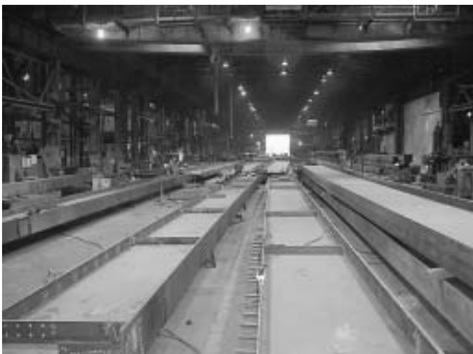
Au Dragon Forgé offered an up-close look at fabricating welded beams for bridges. ADF operates in the former Dominion Bridge Co. works.
