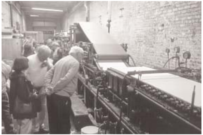
Examining the 1947 Fourdrinier machine at St. Armand Paper.
