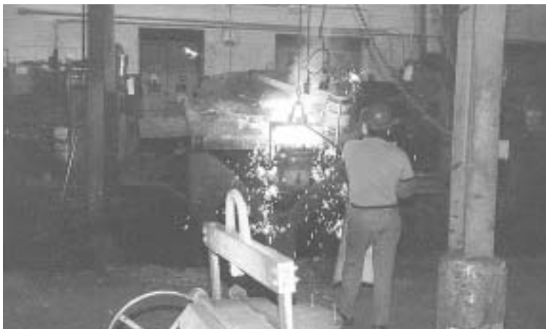
Belcher Foundry—filling a transfer crucible. At least one small foundry will be scheduled for the '04 Annual Conference in Providence, June 10-13.
