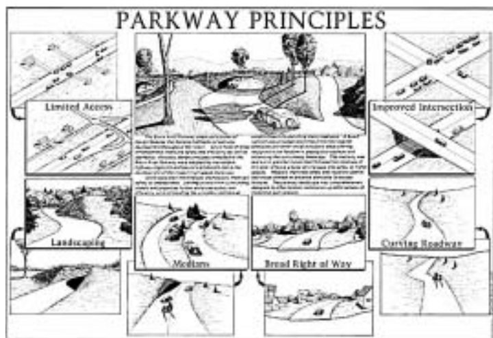
HAER drawing illustrating the roadway geometry and design principles that guided the development of the Bronx River Parkway and made it a landmark in the development of motor roads. HAER No. NY-327.
