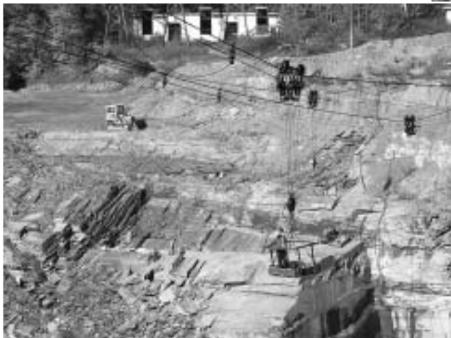
At the Penn Big Bed Slate Quarry, a worker rides the cableway up from the pit.
