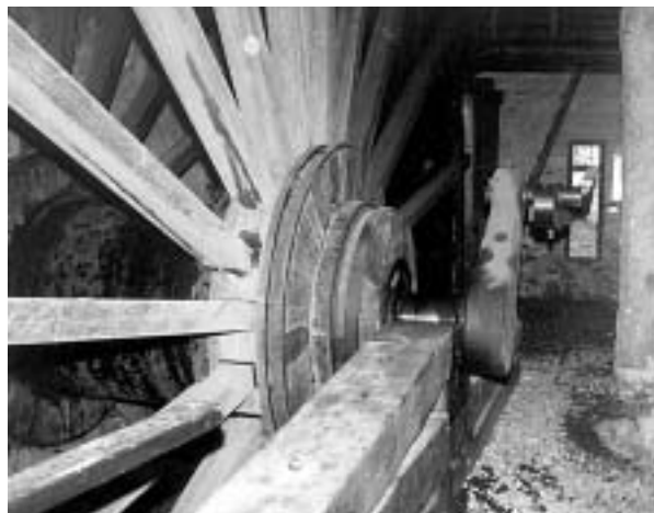
Magnificently reconstructed, the waterwheel at Pershyttan drives the stångång (left), which once transmitted power for pumping to nearby mines by means of reciprocating rods.
