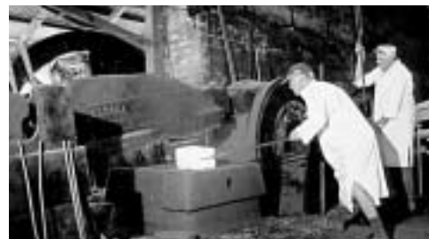
Working the Lancashire forge at Karmansbo: The heated iron is lifted from the hearth onto a small cart (left), transferred to the “mumblingshammer” (middle), then to the rolling mill (right).
