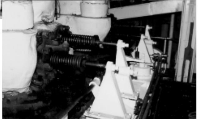
*Midsection of the Badger's port engine, between the (upper) high-pressure cylinders and (lower) low-pressure cylinders, showing the bell cranks that operate the steam valves.*
